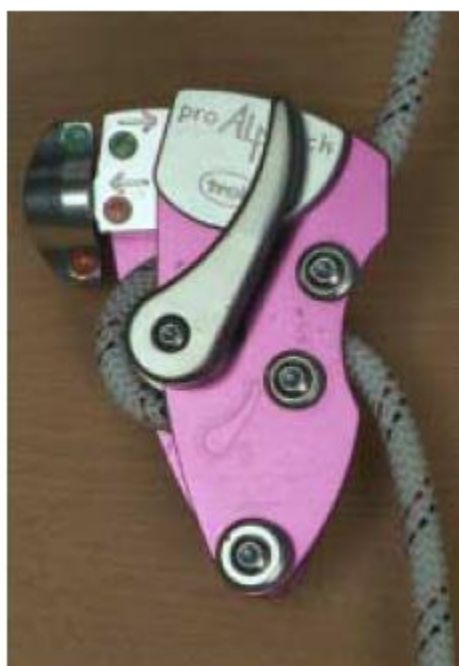
Figure 47 Troll pro Allp tech Type C descender
