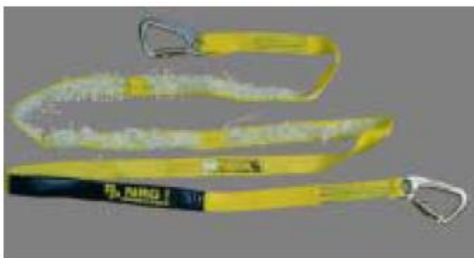
Figure 51 Pammenter & Petrie 'NRG' lanyard (shown after test)
